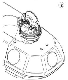
Disconnect the wires from the lamp contacts and insulate the fastons, as power is still present and could cause a short circuit
