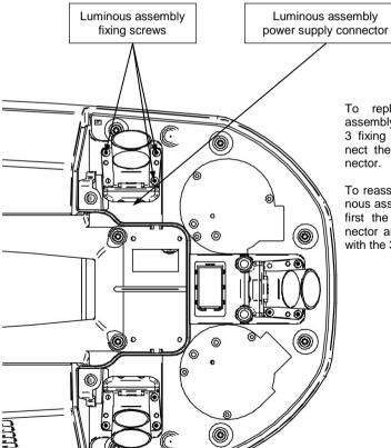
To replace the luminous assembly firstly unscrew the 3 fixing screws and disconnect the power supply connector.
