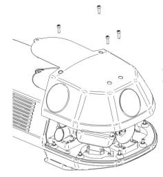
To access the luminous assembly unscrew the dome blocking screws and remove the dome upwards as shown in the drawing.
