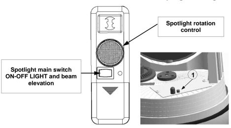
By pressing the main switch once, the spotlight is ON and ready to work. It is then possible to control and direct the light where required. Press the main switch a second time to turn the spotlight OFF. The spotlight will then return to the rest position.
