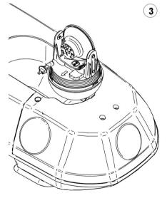
Do not touch the glass bulb with bare fingers when replacing the bulb Refasten the spring support and reconnect the wires to the contacts.
